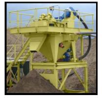
The CDI F-Range offer sand processing solutions that utilize cyclone, pump and dewatering technology to produce specification sands and are capable of recovering all saleable sand coarser than 40 micron therefore increasing sand production, increasing plant capacity and reducing settling pond maintenance costs. Nearest Dealer / Agent: Contact CDI for details. (currently enlisting in sellect countries)
